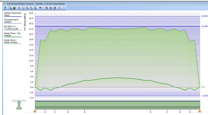
Figure C.13 Stresses at transfer when curing at 28 celsius
